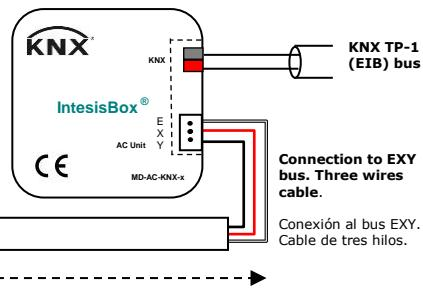
**IMPORTANT:** If the MD-AC-KNX-1B/16/64 gateway is **not** placed at one end of the EXY bus, the terminal resistor should be deactivated. Remove Jumper 1 in order to deactivate the  $120\ \Omega$  terminal resistor.
